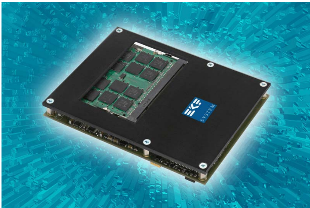
XB1 COM Express Module with Heatspreader
